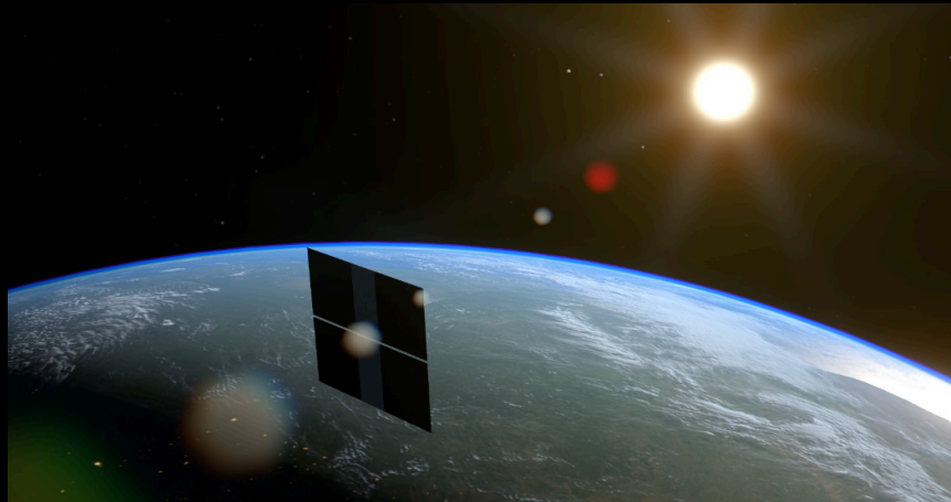
Figure 3. A data center in Sun Synchronous Orbit, showing a 4km x 4km deployed solar array and radiators.
